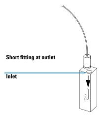
Figure 42 Connecting Tubing to Flow Cell
