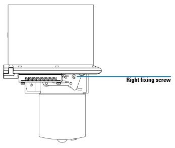
Figure 31 Top View of the Multicell Transport in Spectrophotometer
