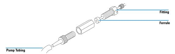
Figure 43 Connecting Tubing to Pump
