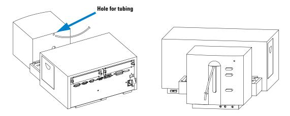
Figure 45 Installing Tubing in the Spectrophotometer
