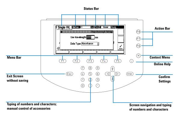
Figure 14 Description of Control Module Keys
