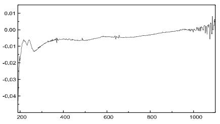
Figure 13 Example of a Blank on Water with Bubbles Causing a Poor Baseline
