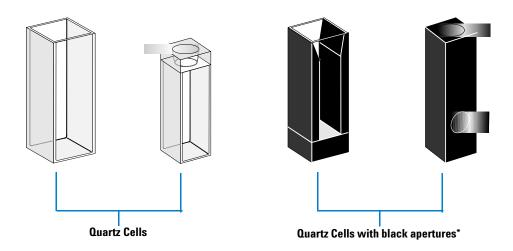
Figure 8 Recommended Cells
