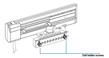
Figure 36 Removing the Cell Holder Assembly
