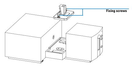
Figure 2 Mounting the Cell Holder
