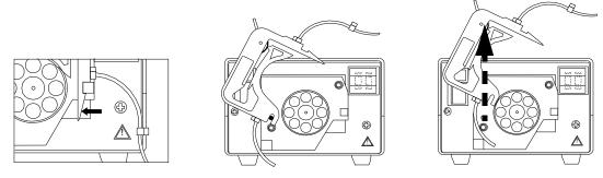
Figure 39 Removing the Tubing Cassette
