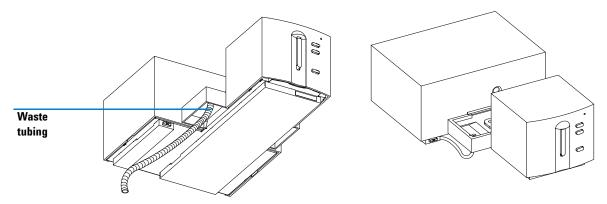
Figure 1 Connecting the Waste Tubing
