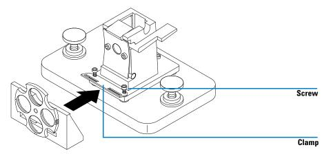
Figure 29 Installing the Optical Filter Wheel Assembly
