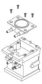
Figure 22 Installing the Cell Stirring Module
