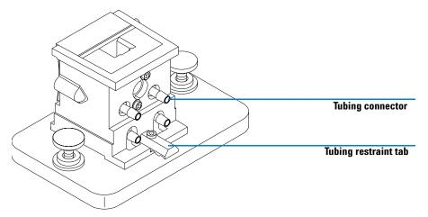
Figure 20 Thermostattable Cell Holder
