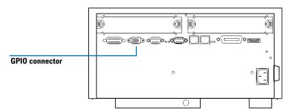
Figure 38 Connector at Rear of Spectrophotometer
