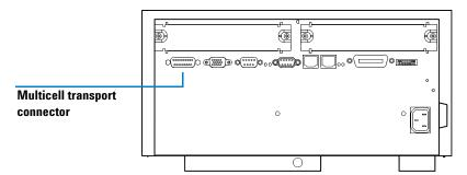
Figure 32 Connector at Rear of Spectrophotometer
