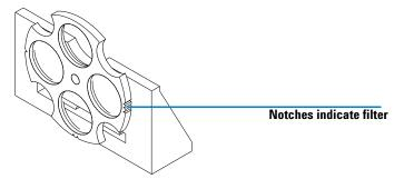
Figure 27 Optical Filter Wheel Assembly
