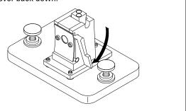
Small volume flow cells and particularly any cells with less than a 2 mm aperture may require use of the optional adjustable cell holder. The adjustable cell holder helps you ensure the cells are properly centered in the light path.
