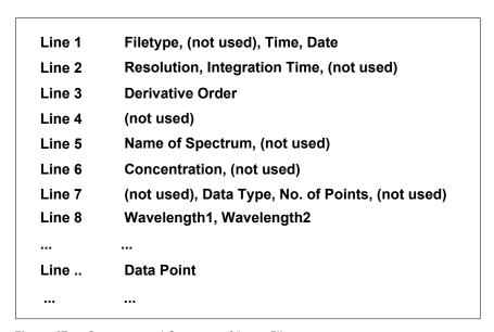
Figure 47 Structure and Contents of \*.wav Files
