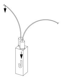
Figure 44 Connecting Tubing to Flow Cell
