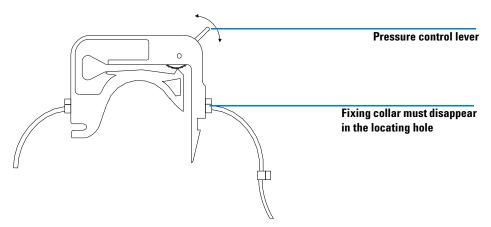
Figure 40 Tubing Cassette with Pump Tubing
