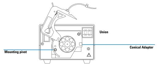
Figure 41 Replacing the Tubing Cassette
