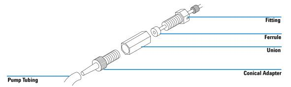
Figure 46 Connecting Waste Tubing to Pump
