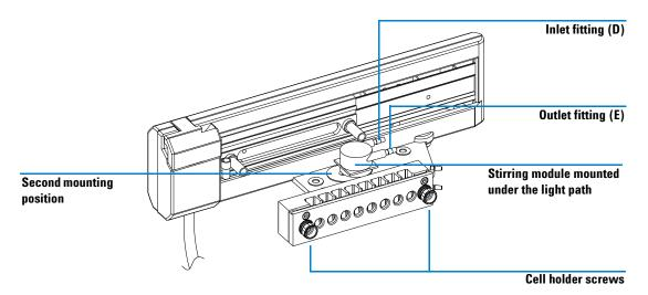
Figure 33 Mounting the Stirring Assembly
