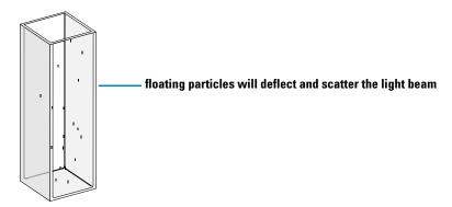
Figure 10 Floating Particles in a Cell
