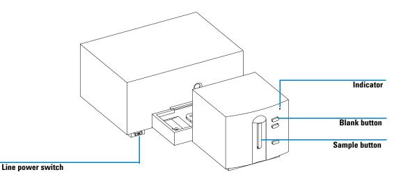
Figure 5 Turning on the Agilent 8453E UV-visible Spectroscopy System
