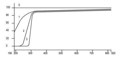
Figure 28 Transmission Characteristics of Filter Wheel Filters
