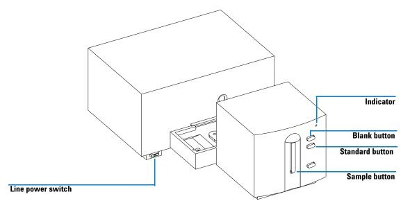
Figure 15 Front View and Keys of the Spectrophotometer
